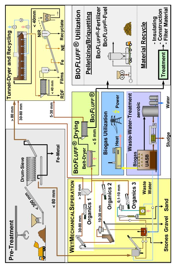
Figure 3: Process scheme total
